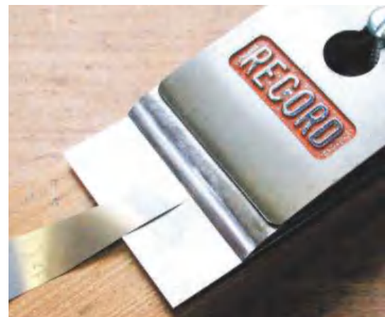
▲ Pic.1 I've made a jig that lets me check the cap iron's fit while under pressure
